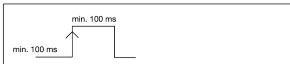
For reset an ESX10-(S)125 in OFF condition a pulse of a duration of min. 100 ms. The ESX10-(S)125 cannot explicitly be switched off.
